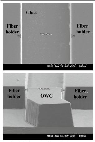
$\textbf{Fig. 2} \ \ \textbf{The FE-SEM photograph of fabricated OWG}$
