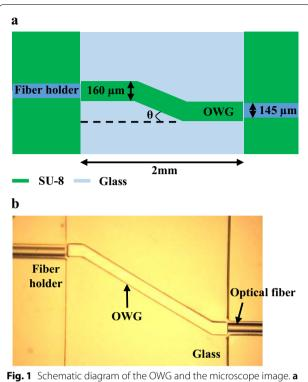
**Fig. 1** Schematic diagram of the OWG and the microscope image. **a** Design values and **b** fabricated SU-8 OWG are indicated
