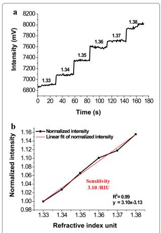
**Fig. 5** The measurement result. **a** LSPR intensity changes according to increase of refractive indices. **b** The amount of increased intensity per refractive index unit. The intensities are normalized as reference to the signal at 1.33
