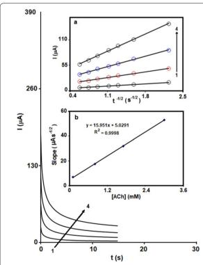
**Fig. 4** Chronoamperograms obtained at MCSNP/SPE in 0.1 M PBS (pH 7.0) for different concentration of ACh. The numbers 1–4 correspond to 0.1, 0.8, 1.7 and 3.0 mM of ACh. Insets: Plots of I vs. t $^{-1/2}$  obtained from chronoamperograms 1–4 (**a**), and plot of the slope of the straight lines against ACh concentration (**b**)
