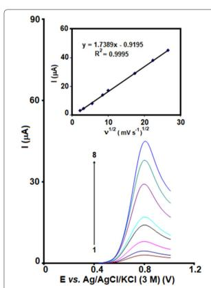
**Fig. 2** LSVs of MCSNP/SPE in 0.1 M PBS (pH 7.0) containing 20.0 μM ACh at various scan rates; numbers 1–8 correspond to 5, 10, 30, 70, 100, 300, 500 and 700 mV s<sup>-1</sup>, respectively. Inset: Variation of anodic peak current vs. square root of scan rate
