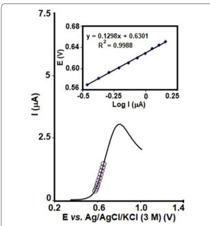
Fig. 3 Tafel plot derived from LSV of MCSNP/SPE in 0.1 M PBS (pH 7.0) containing 20.0  $\mu$ M ACh at scan rate of 5 mV/s
