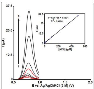
**Fig. 5** DPVs of MCSNP/SPE in 0.1 M PBS (pH 7.0) containing different concentrations of ACh (0.1, 2.5, 8.0, 20.0, 60.0, 100.0, 300.0 and 500.0  $\mu$ M). Inset: The plot of the peak current as a function of ACh concentration in the range of 0.1–500.0  $\mu$ M
