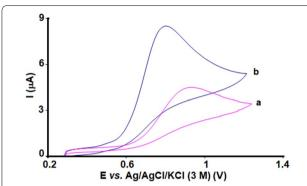
**Fig. 1** CVs of (a) unmodified SPE and (b) MCSNP/SPE in the presence of 90.0  $\mu$ M ACh at pH 7 (at 5 mV s<sup>-1</sup>)
