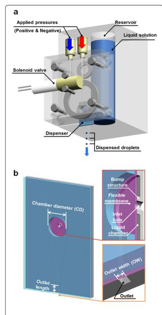
Figure 1 Schematics of a pneumatic dispensing system: (a) overview of the system and (b) design of the dispenser.
