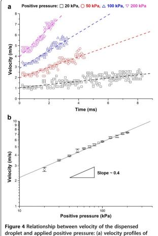
Figure 4 Relationship between velocity of the dispensed droplet and applied positive pressure: (a) velocity profiles of the dispensed droplets (dash lines are linear fitting curves for each applied positive pressure) and (b) The relationship between velocity and positive pressure (velocities were exponentially increased to positive pressure).
