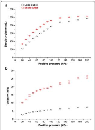
Figure 7 Comparison of two different outlet lengths: plots of (a) droplet volume and (b) velocity vs. positive pressure.
