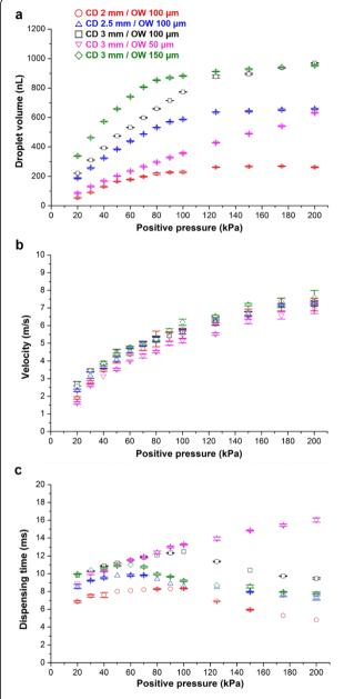
**Figure 5** Characterizations of the dispensing system with various design parameters: plots of (a) droplet volume, (b) droplet velocity, and (c) dispensing time vs. positive pressure.
