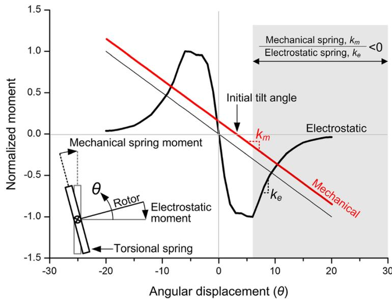
**Figure 2** Normalized mechanical and electrostatic moment of the AVC-driven microscanner with respect to the angular displacement. The electrostatic moment (bold black curve) is calculated by FEA, and a unit comb electrode set is used to account for the fringing fields. The mechanical restoring moment of the torsional spring is depicted for the torsional spring with (red line) and without (thin black line) an initial tilt angle.
