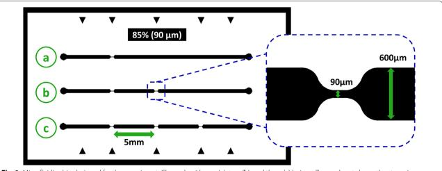
Fig. 1 Microfluidic chip designed for the experiment. Channels with one (a), two (b), and three (c) lesions. Zoomed part shows the stenosis geometry and sizes
