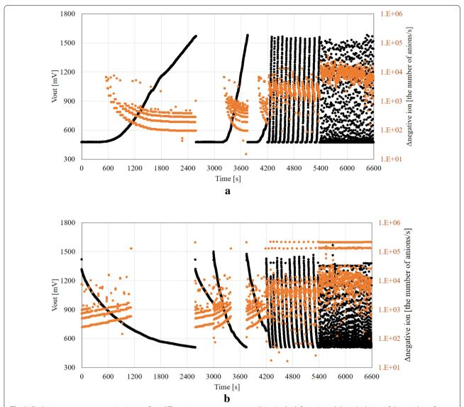
**Fig. 3** Real-time response to negative ions in four different ion concentration condition in the left y-axis and the calculation of the number of negative ions adsorbed on the extended gate electrode per second in the right y-axis; **a** p-type nanoFET device, **b** n-type nanoFET device
