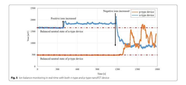
ion balance in real-time at the antistatic target position, where is affected by the ion blower.
