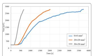
**Fig. 4** Real-time measurement results of negative ion detection in the air depending on the size of the extended gate electrode of the nanoFET sensor
