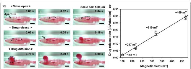
**Fig. 3** a The sequential images show the drug release process of the proposed magnetic micropump with a short exposure (less than 1 s) of magnetic field (469 mT), including the valve opening, the drug release, and the drug diffusion. **b** The quantitative evaluation of the drug release according to the strength of the magnetic field from 152 to 469 mT. Error bars indicate the standard deviation (n = 10)
