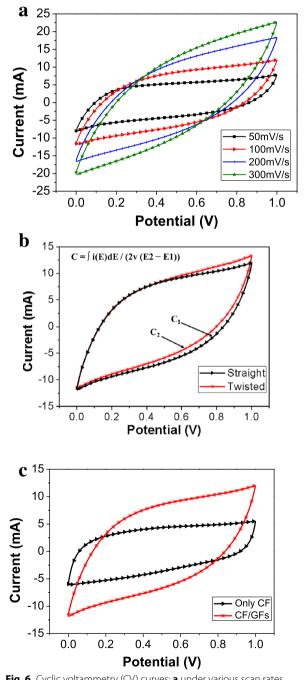
**Fig. 6** Cyclic voltammetry (CV) curves: **a** under various scan rates, comparison between **b** straight and twisted position, and **c** before and after being coated with GFs at the scan rate of 100 mV/s
