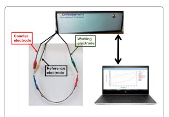
**Fig. 5** Test setup for the electrochemical analysis of the fabricated supercapacitor
