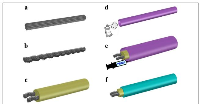
**Fig. 2** Fabrication sequences of the proposed flexible cable-shaped supercapacitor: **a** deposition of GFs on the surface of the CF bundles, **b** 20 times twisted CF bundles, **c** deposition of gel electrolyte, **d** spraying of release agent, **e** injection of PDMS, and **f** removal of the shrinkable tube
