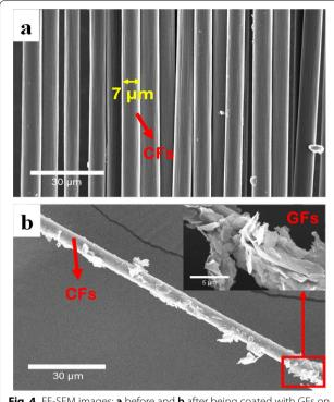
**Fig. 4** FE-SEM images: **a** before and **b** after being coated with GFs on the surface of CFs
