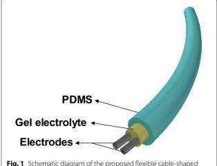
**Fig. 1** Schematic diagram of the proposed flexible cable-shaped supercapacitor
