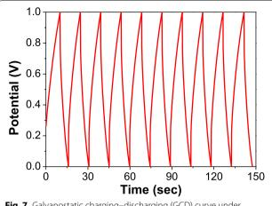
**Fig. 7** Galvanostatic charging–discharging (GCD) curve under current of 10 mA
