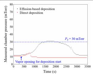
**Fig. 1** Variation of the recorded machine chamber pressure along with time in the present effusion-based deposition and direct deposition processes. In the depositions, the target thicknesses were both 30 nm
