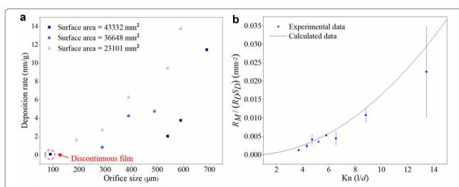
Fig. 3 Deposition outputs. a The deposition rates in different chambers with different orifice sizes, and b comparison of the experimental results and the model, calculated by Eq. (7)
