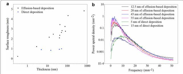
**Fig. 5** Surface roughness of the direct deposition and the present effusion-based ultra-thin Parylene deposition measured by AFM surface scanning (a) and according power spectral density (b)
