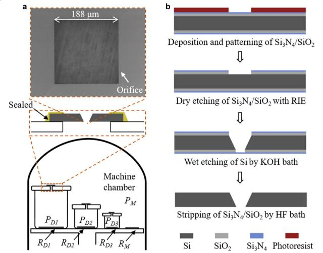
Fig. 2 Working principle of the present ultrathin Parylene deposition (effusion-based deposition). a The schematic of deposition system with a typical SEM image of the microfabricated orifice. b Schematic of the fabrication process of the orifice chip
