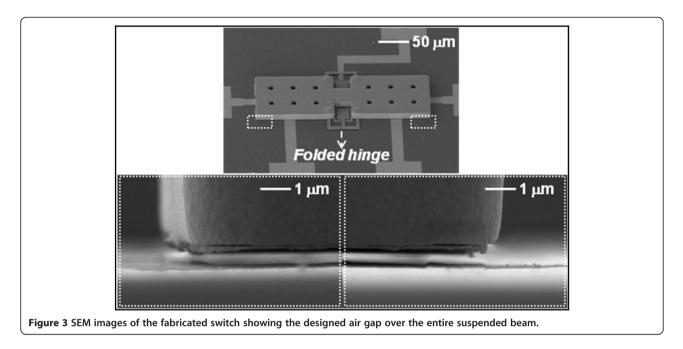
could achieve an air gap thickness as designed (0.45  $\mu$ m) over the entire suspended structure, shown in Figure 3.
