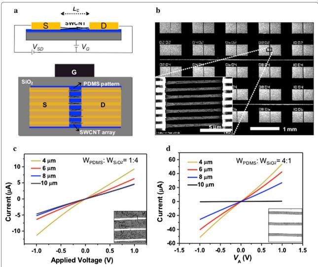
**Fig. 5 a** Schematic layout of SWCNTs-FET device. **b** Large-area SEM image of the device with highly oriented nanotube bundles. The *inset* shows an enlarged view of a unit device. **c**, **d** Electrical characteristic of the device with various channel lengths ( $L_c$ ) and two different pattern geometries: **c**  $W_{PDMS}$ : $W_{SiO_2} = 1:4$  (500 nm:2000 nm) and **d** 4:1 (2000 nm:500 nm). *Inset* AFM images of aligned SWCNTs
