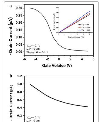
**Fig. 6** A typical gating effect of the devices with **a** highly oriented nanotube bundles [ $L_c=10~\mu m,W_{PDMS}:W_{SiO_2}=4:1~(2000~nm:500~nm),$  VDS = -0.1~V]. The *inset* shows output characteristics of the device, for three gate voltages (VG = -5, -10, and -15~V), measured in steps of 0.5 V. **b** FET device with Lc of 10  $\mu m$ , based on SWCNT membrane (VDS: -0.1~V). The device exhibits a turn-off ratio less than  $\sim 10$
