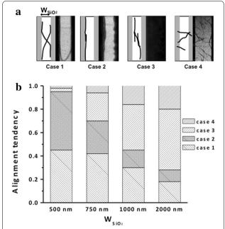
Fig. 4 a Four representative categories of the SWCNTs alignment. **b** Phase map of alignment tendency with varying widths of the hydrophilic region ( $W_{SiO_2}$ ) for a given concentration (~0.1 mg/ml). As shown, the degree of alignment was decreased with increasing the hydrophilic region (from case 1 to case 4)
